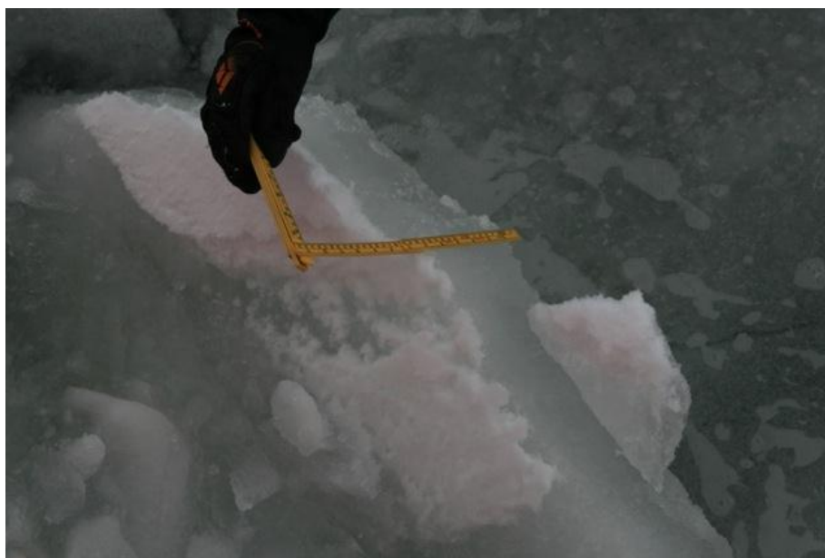
Figure 4 Measuring thickness of newly broken ice (Kraft Johansen)
